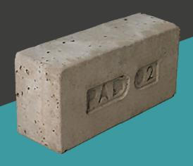
Supreme padstones are high strength dense concrete blocks designed to support the weight of load-bearing lintels whose ends rest on the padstone. The concrete used in the manufacturing of the padstone conforms to a compressive strength class C40/50.
